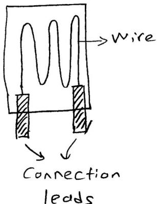
when strain occurs its resistance R changes, Fractional changes in R is proportional to strain  $\epsilon$
