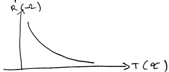
$$R = R_0 e^{\beta \left( \frac{1}{T} - \frac{1}{T_0} \right)}$$
